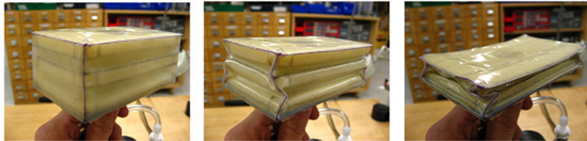
Figure 2 Ideal flat top surface during deflation
